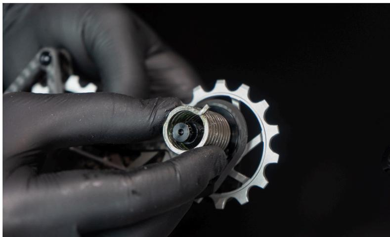
9. Place the seal on the spring in the same direction shown in the photo.
