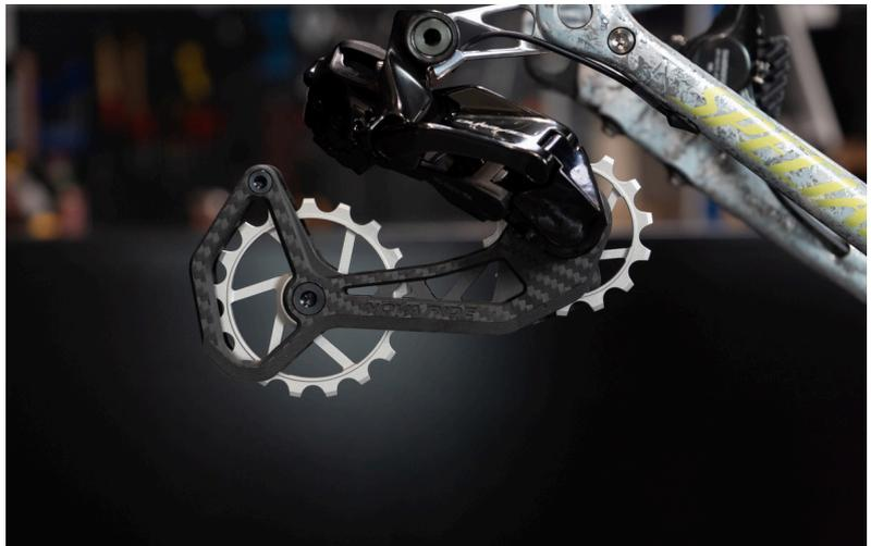
**11.** Your chain length will change because the Nova Ride pulleys are larger. It is therefore highly recommended to use a new chain. **We strongly recommend adding 2-4 links compared to your previous chain.**
