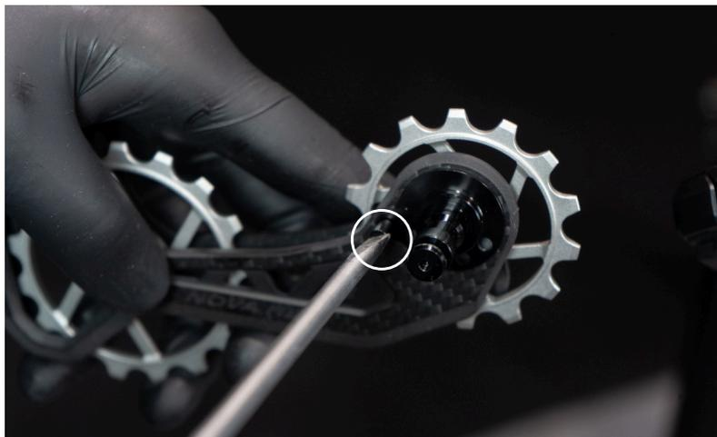
8. Take your Nova Ride derailleur hanger and insert the spring into the middle tension hole as pictured.
