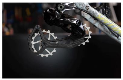
11. Your chain length will change because the Nova Ride pulleys are larger. It is therefore <u>highly</u> <u>recommended</u> to use a new chain. We strongly recommend adding 2-4 links compared to your previous chain.
