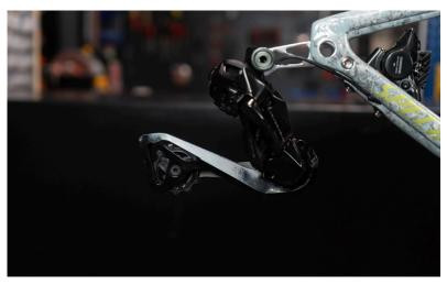
**4.** Unscrew the derailleur screw using a T10 Torx key while firmly holding your original cage.
