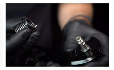
7. Take your Nova Ride derailleur hanger and unscrew the stopper circled in white using a flathead screwdriver.
