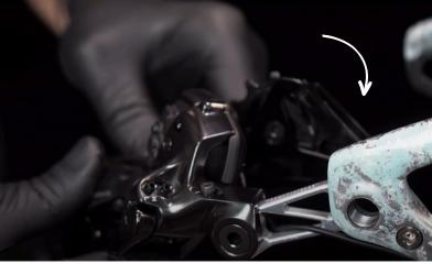
6. Once there is no more tension, remove the original cage from the derailleur and keep the seal and spring for steps 8. and 9.
