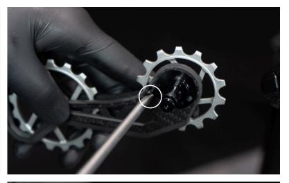
**8.** Take your Nova Ride derailleur hanger and insert the spring into the middle tension hole as pictured.
