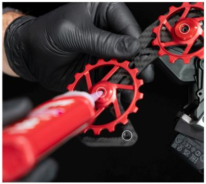
**21.** Screw back the two 2,5 mm hex key screws, and the one 2 mm hex key screw.
