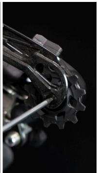
**5.** Loosen but do not remove completely the main central nut with the Nova Ride tool and a 5 millimeters hex key.
