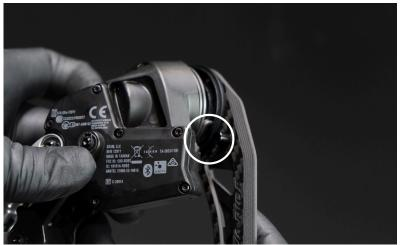
**15.** Rotate the cage clockwise, hovering over the D interface while passing over the derailleur stop.
