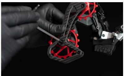
**22.** This spacer moves the derailleur from the frame and allows to reach the right positon of the cage compare to the cassette.
