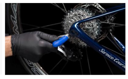
**4.** Unscrew the two wheels from the Sram derailleur cage with a 2,5 millimeters allen key.
