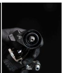
**13.** Place the spring into the original derailleur body.
