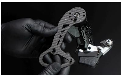
**19.** Then reinstall the 14T pulley wheel on the upper part of the cage and the 17T pulley wheel on the lower part.
