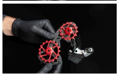
**20.** Apply threadlock inside of each of the three black screw holes.
