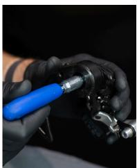
**6.** Rotate the stock front cage counterclockwise until there is no more tension, then remove the central nut and the original cage.
