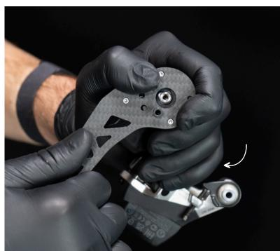
**16.** Tighten the nut, by hand first with the Nova Ride tool provided.
