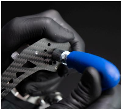
**18.** Put back the two custom black screw (3 and 4 mm hex key) on the carbon front cage.
