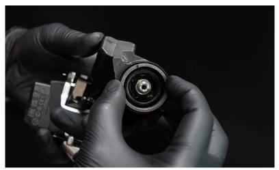
**14.** Take your Nova Ride carbon front plate and insert the spring into the middle tension hole in the axle as pictured.
