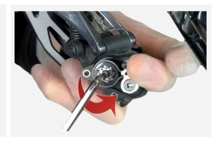
**2.** Hold the Shimano cage firmly and twist it clockwise to remove it.
