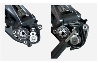
**1.** Unscrew the central axle by using the 4mm Allen key.
