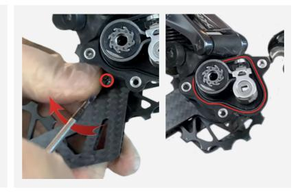
**2.** Replace the cover and screw the 3 screws using the 2mm Allen key.
