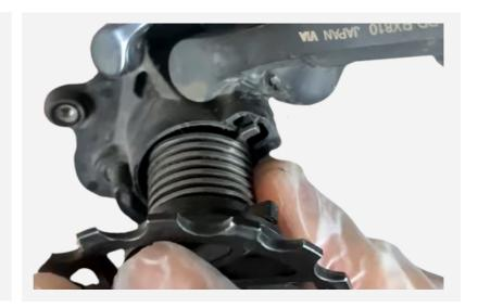
**2.** Hold the cage securely in the derailleur and screw the central axle by using the 4mm Allen key.
