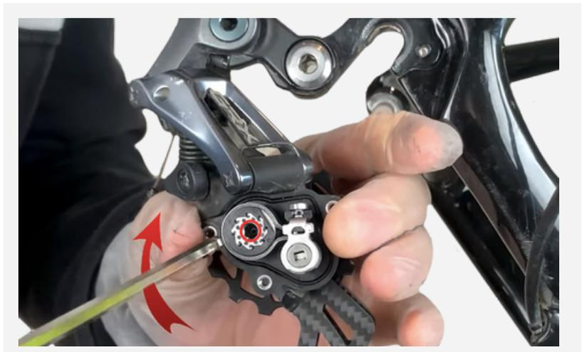
3. Rotate the cage counter-clockwise to tension it.
