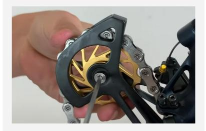
**2.** Remove the second pulley wheel by using the 5mm Allen key.
