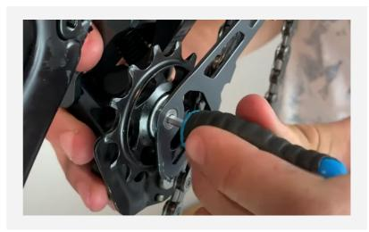
**3.** Replace the second standard pulley with the second Nova Ride pulley and screw the pulley back on with the same screw.
