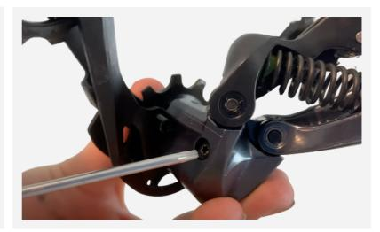
**5.** Hold the Shimano cage firmly and twist it clockwise to remove it.
