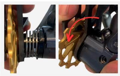
**3.** Rotate it until the stopper (circled in red) comes up against the derailleur (blue line).
