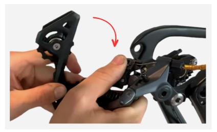
**1.** Once there is no more tension, remove the derailleur cage. Save the spring and the seal for later.
