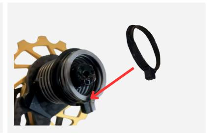
**2.** Put the Nova Ride CCD in the derailleur and rotate it counterclockwise as pictured.
