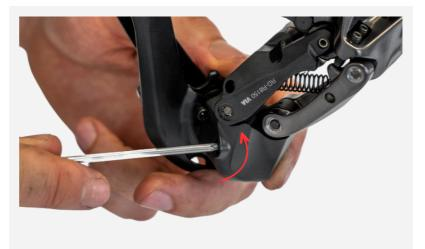
**5.** Hold the Shimano cage firmly and twist it clockwise to remove it.
