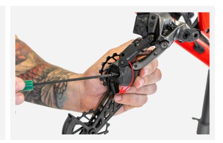
**2.** Screw the stopper back on, with a little of Loctite, by using the flat screwdriver.
