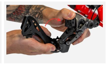
**1.** Once there is no more tension, remove the derailleur cage. Save the spring and the seal for later.
