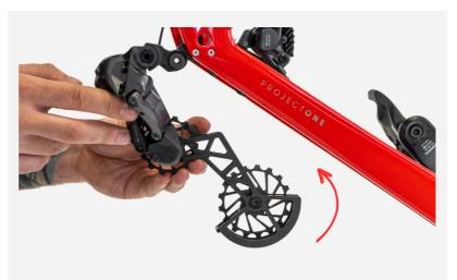
**3.** Rotate the Nova cage until you see the stopper screw pitch (circled in red).
