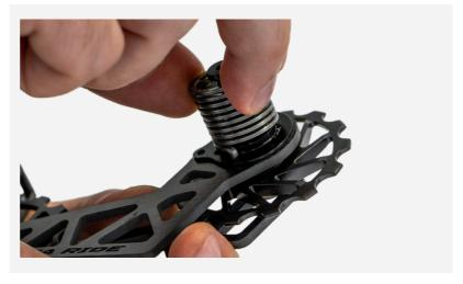
**1.** Put the seal on the spring in the same direction as in the photo.
