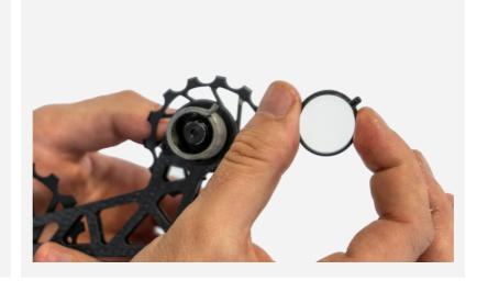
**2.** Put the Nova Ride CCD in the derailleur and rotate it counterclockwise as pictured.
