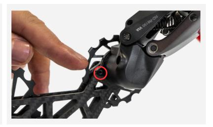
**1.** Reinstall the original derailleur screw by using the Torx key.
