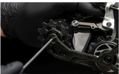
**4.** Unscrew the lower stock pulley also with a 2,5mm Hex Allen key.
