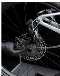
**3.** First unscrew the lower stock pulley using a T25 Torx Key.
