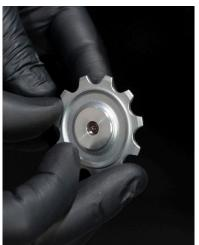
**8.** Screw the pulley back on with the same screw.
