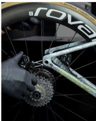
**3.** First unscrew the lower stock pulley using a 3mm Hex Allen key.
