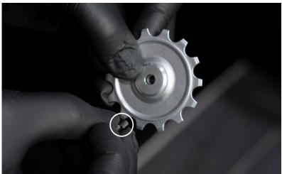
**7.** Insert and screw the pulley on with the same screw.
