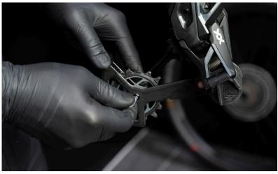
**4.** Unscrew the upper stock pulley also with a T25 Torx key.
