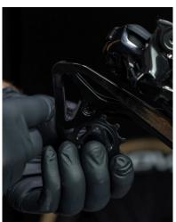
**4.** Unscrew the upper stock pulley also with a 3mm Hex Allen key.
